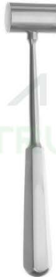
Mead Mallet 10-588 19cm Head diameter 26.0mm Weight 11 oz 315 grams Head Weight: 6 oz 170 grams
